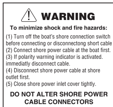
Shore Power Connection
