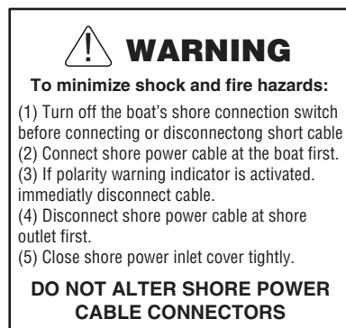
Shore Power Connection
