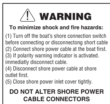
Shore Power Connection
