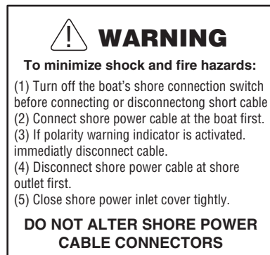
Shore Power Connection
