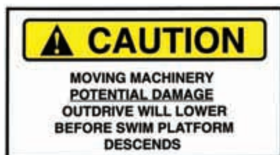
Above Hydraulic Swim Platform Switch
