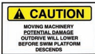
Above Hydraulic Swim Platform Switch
