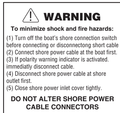
Shore Power Connection
