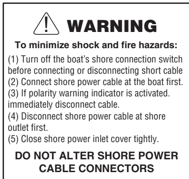
Shore Power Connection
