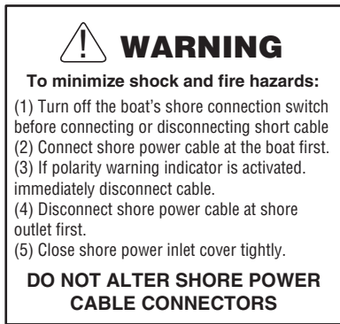
Shore Power Connection
