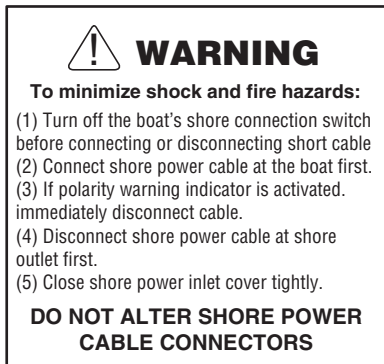
Shore Power Connection
