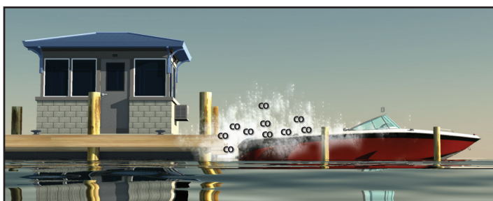
Blockage of boat exhaust by obstruction.
