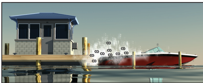
Blockage of boat exhaust by obstruction.
