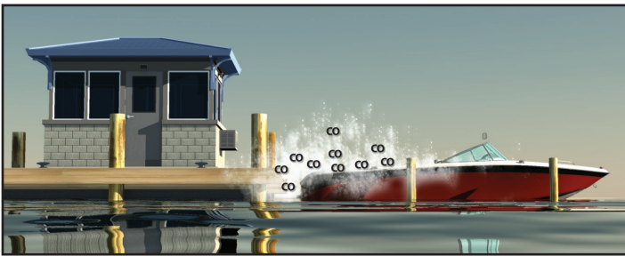
Blockage of boat exhaust by obstruction.
