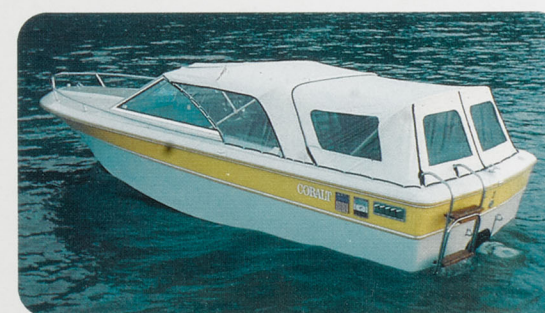
Camper Top: For overnights. Ample headroom and visibility, zippers to top canvas and snaps to deck.
