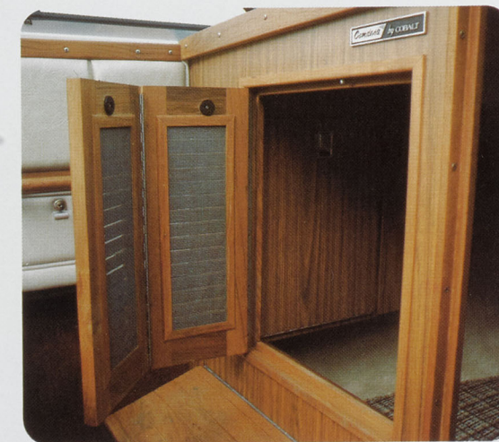
Pass Thru Door enhances openness of cabin area on the port side. Doors are lockable and have insect screens on the cabin side.
