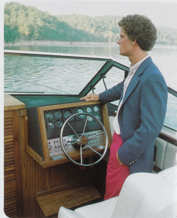
Control Center instrumentation is complete with speedometer, tachometer, ammeter, oil pressure and temperature gauges and trim indicator. Clock with sweep second hand and cigarette lighter are also included. All function switches are coupled to individual indicator lights and circuit breakers. Ash tray and drink holder are mounted in teakwood surround.
