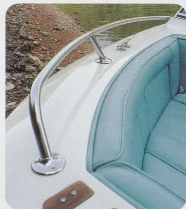
Bow Rails and fittings are polished stainless steel with welded stanchions solidly mounted into die threaded metal, molded into underside of deck.
