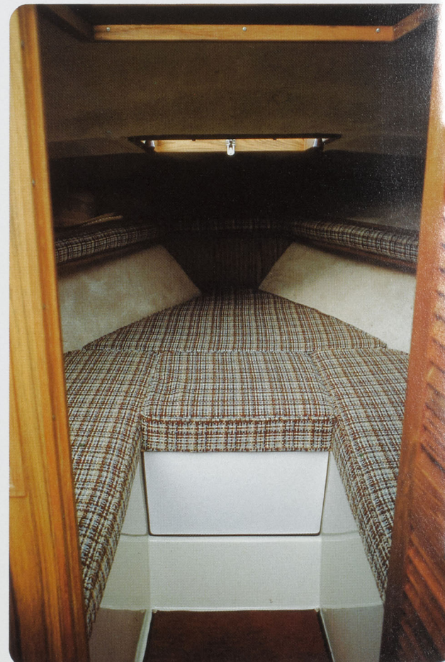
Cabin features spacious V-berths for those overnight outings. Four piece cushion ensemble is upholstered with vinyl on reverse side. Cushions are easily raised for access to storage areas beneath. An insert cushion covers floor area for sleeping. Teak trimmed side shelves on both sides extend all the way forward and allow extra space for small item storage.
