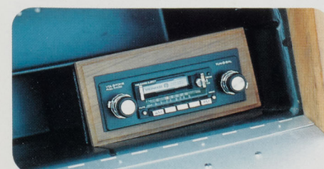
Stereo: 8 Track or Cassette, AM/FM radio with power antenna (mounts in glove compartment on runabout models).
