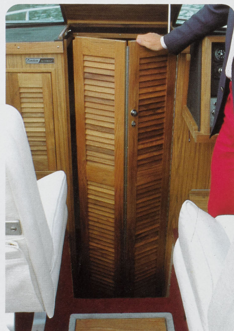
Companionway Doors are solid teakwood and louvered for ventilation. Full length piano hinge break doors in the center. Hook latch secures them open. Lockable when closed and fitted with insect screens on the cabin side.
