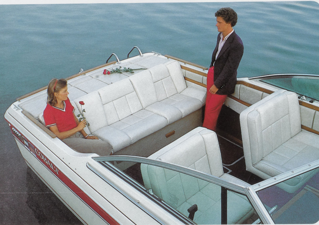
Seating includes extra wide Captain's chairs, providing enough room for two people comfortably. Driver's seat is adjustable fore and aft. Spacious stern seat, covers full breadth of aft area. Easily unlatched to slide forward for immediate access to engine compartment. When folded down flat, the seat may be utilized as an extra berth.
