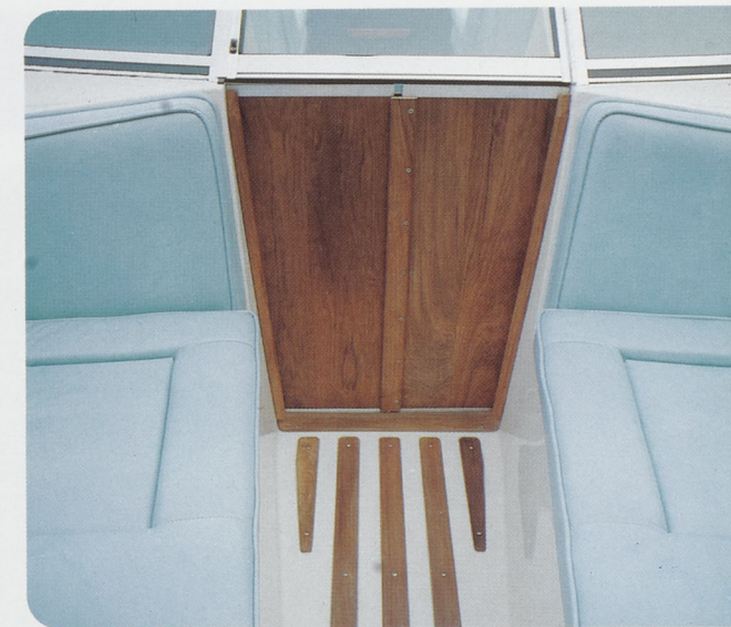
Walk Thru in bowrider models features handcrafted solid teakwood walk thru doors. Capped top and bottom with metal and triple hinges for added strength. Doors swing aft and bolt latch closed. Friction catches keep them firmly in the open position. Steel yolk molded into deck adds additional strength to avoid flex in this area.
