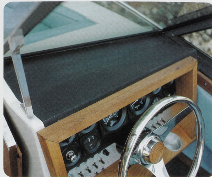
▲ Anti-reflection surface on deck area above control panel is flat black to eliminate glare and reflection from windshield.
