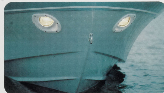
Docking Lights: Sealed beam bright and flush mounted on each side of hull bow. 19's and Condesa.
