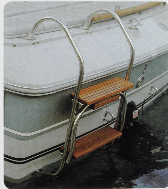
Boarding ladder is stainless steel and wraps over deck. Steps are solid grooved teakwood for slip resistance. Fold down section affords easy entry into boat from the water.
