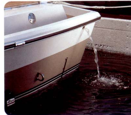
Recessed deck is self-draining by way of thru-hull fittings.
