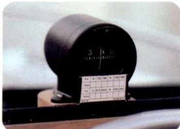
Compass for bow rider models is aircraft type; mounts above steering wheel on dash.
