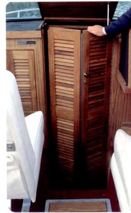
Companionway Doors are solid teakwood and louvered for ventilation. Hook latch secures them open. Lockable when closed and fitted with insect screens on the cabin side.
