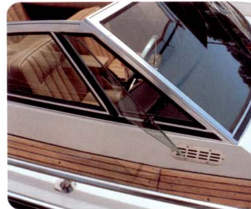
Curved, welded, single piece windshield with vented side wings for ventilation.
