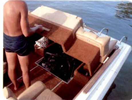
Motor box and jump seats are built into a single unitized unit that raises from floor level with the help of assist cylinder.
