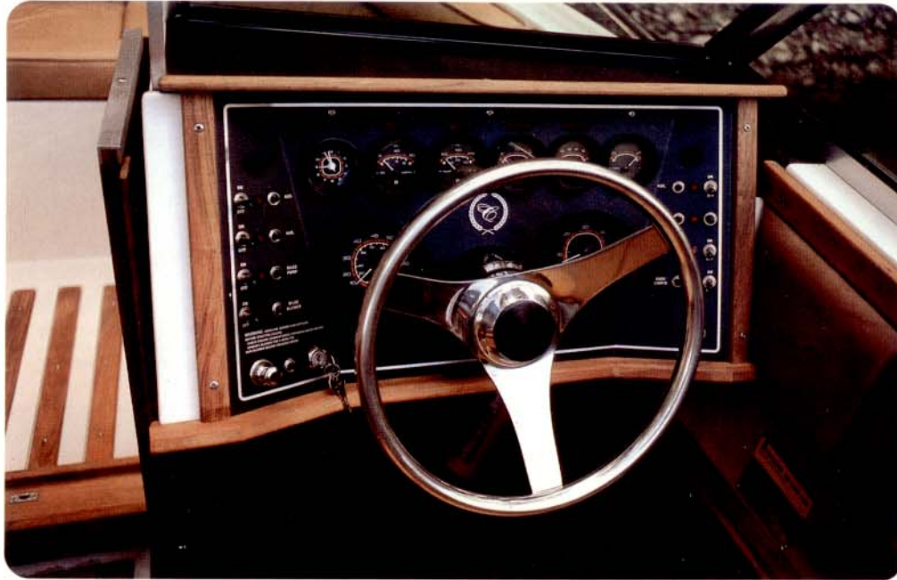
Control panel is aluminum with teak trim. Three section, concave design includes total instrumentation; switches, indicator lights, warning lights and circuit breakers. Top of dash is flat black to avoid reflection and glare.
