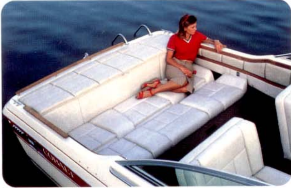
Spacious stern seat, covers full breadth of aft area. Easily unlatched to slide forward for immediate access to engine compartment. When folded down flat, the seat may be utilized as an extra berth.
