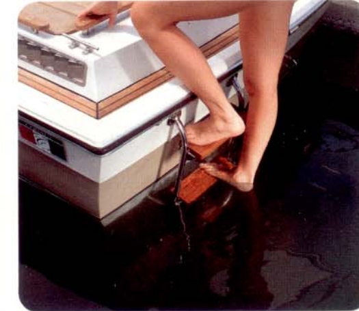
Boarding ladder with thin profile has fold down step for easy entry from the water.
