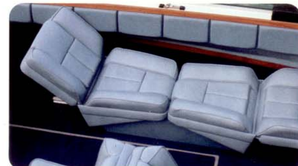
Sleeper seats are easily converted to lounge and sleeper positions with specially designed mechanism in base.
