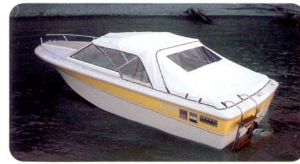
Stern curtain: Fastens to top canvas with zipper and snaps to deck for complete cockpit enclosure.
