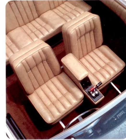
Central seating with shift and throttle controls mounted in between, on storage/armrest console.
