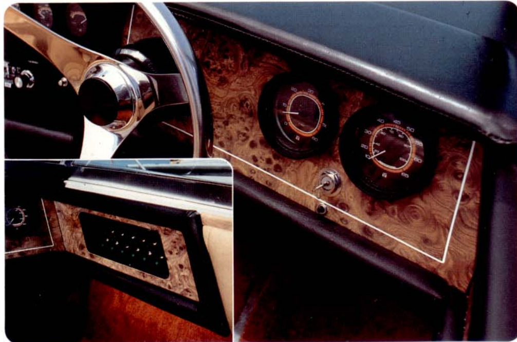
Speedometer and tachometer are located to right of steering wheel with key ignition below. Indicator lights with respective switches and resettable breakers are recessed in drivers side panel.
