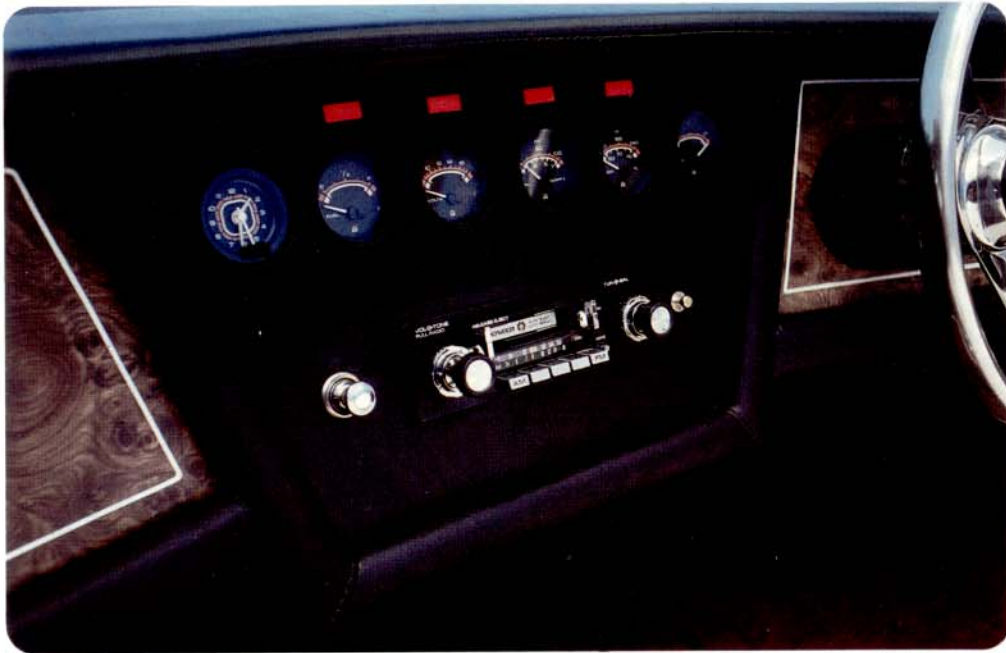
Instrument panel in center of dash includes voltmeter, oil pressure, fuel, temperature, trim indicator and clock. Four warning lights across top for oil pressure, water temperature, low fuel and low voltage. Cigarette lighter and horn button on each side of optional stereo tape deck opening.
