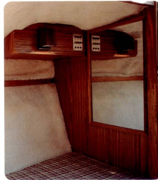
Lighting Control Panel inside cabin on starboard bulkhead, contains switches for cabin interior, engine and floor storage lighting.
