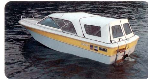
Camper Top: For overnights. Ample headroom and visibility, zippers to top canvas and snaps to deck.
