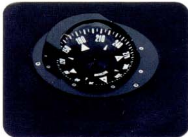
Compass: 5" illuminated bubble style with double axis gimble system for 19CD and Condesa
