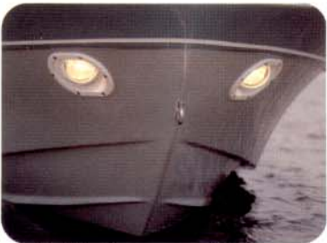
Docking lights are sealed beam bright and flush mounted on each side of hull (19's and Condesa only).
