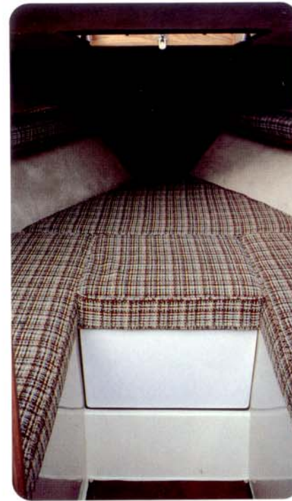
Cabin features spacious V-berths for overnight outings. Four piece cushion ensemble is upholstered with vinyl on reverse side and is easily raised for access to storage areas beneath.
