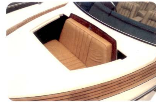
Combination closed deck/bow rider. Deck hatch opens to reveal seating below the deck.
