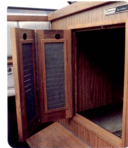
Pass-Thru-Door enhances openness of cabin area on port side. Doors are lockable and have insect screens on the cabin side.
