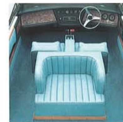
CM-9's mid-engine location allows innovative seating on the motor box cover and forward center of gravity.
