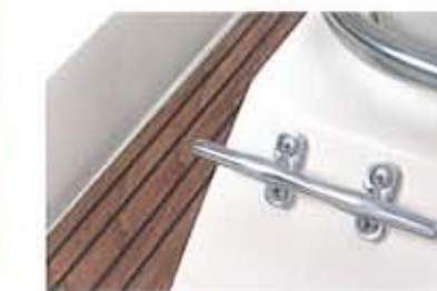
Cleats and other hardware attach to metal plates imbedded in fiberglass.
