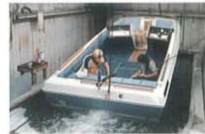
In-plant testing tank is used for final quality check.
