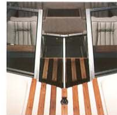
Electrically-operated center windshield section lowers into deck.
