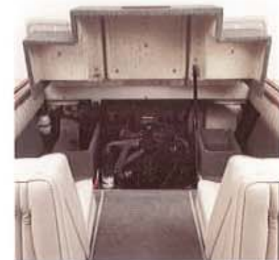
Power assist cylinder raises jump seats and motor box cover as a single unit.
