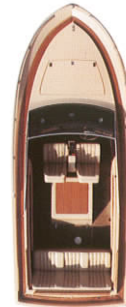
Large, comfortable rear seating area is possible with mid-engine location.
