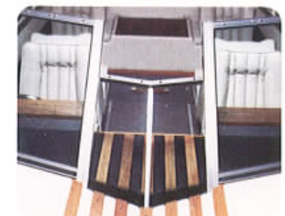
The electrically operated windshield section lowers into the deck.
