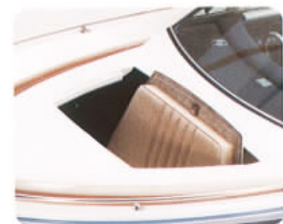
The unique bow seat hatch features a torsion-bar mechanism for easy operation.
