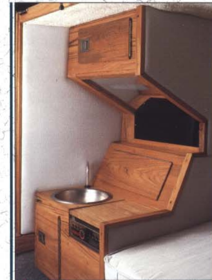
Galley with sink and single-burner alcohol stove (shown on 21CC/ replaces port side chair) .....
