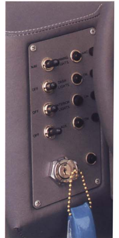
Coated aluminum panels, aircraft circuit breakers, stainless switches, all to insure reliability.
