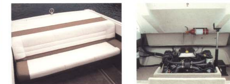
Electrically operated, one piece motor box includes sundeck
