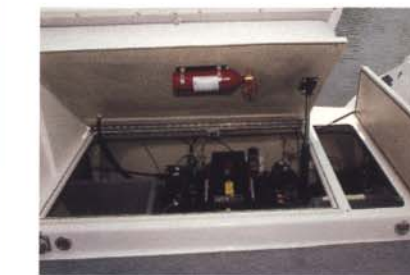
Electric motor box/seating area doubles as storage compartment
