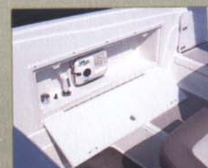
Air Compressor and Transom Shower
