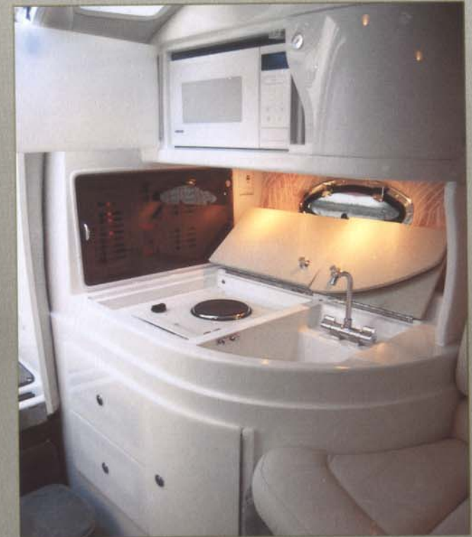
Galley Area w/ Single Burner Electric Stove and Microwave
