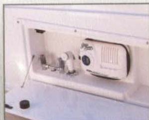
Transom Shower and Air Compressor
