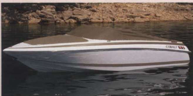
Tonneau Covers - Bow and cockpit covers shown. (Not recommended for long term storage)
