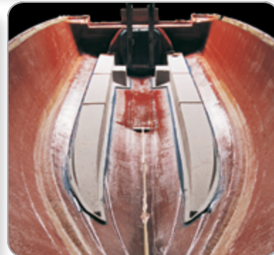
Bonded Fiberglass Stringers
